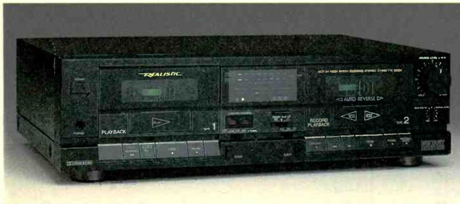
Response:  $\pm 3$  dB: 20-17,000 Hz (metal), 20-16,000 Hz (CrO<sub>2</sub>/Hi-Bias/Type II), 20-15,000 Hz (normal/Type I). **Wow and Flutter:** 0.06% WRMS. S/N: 70 dB Dolby C; 62 dB Dolby B ("A" weighted, metal tape). **Distortion:** 1.0% 3rd HD. **Record/Play Head:** Permalloy. **Erase Head:** Ferrite. **Size:** 5 x 16<sup>1</sup>/<sub>16</sub> x 12<sup>9</sup>/<sub>16</sub>"
