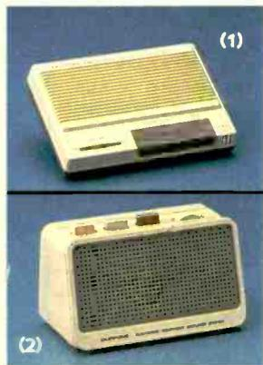
(1) **DUÖFONE-102.** Adds hands-free talking and listening to any phone—just plug in. Features automatic sensitivity adjustment, high-speed talk/listen switching and privacy button to temporarily disable mike.  $2 \times 6\frac{3}{4} \times \frac{3}{4}$ ". Phone-line powered. Jack for AC adapter (#273-1455, extra) for use on low-current phone lines. 43-292 (TSP available) . . . . . 39.95
