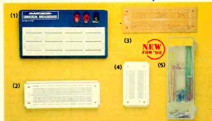
The fast way to design your own circuits! Our breadboards accept a wide variety of devices and make circuit changes as easy as plugging and unplugging wires. When your circuit is working properly, it's simple to transfer it to the matching experimenter's PC board for a soldered, permanent version.
