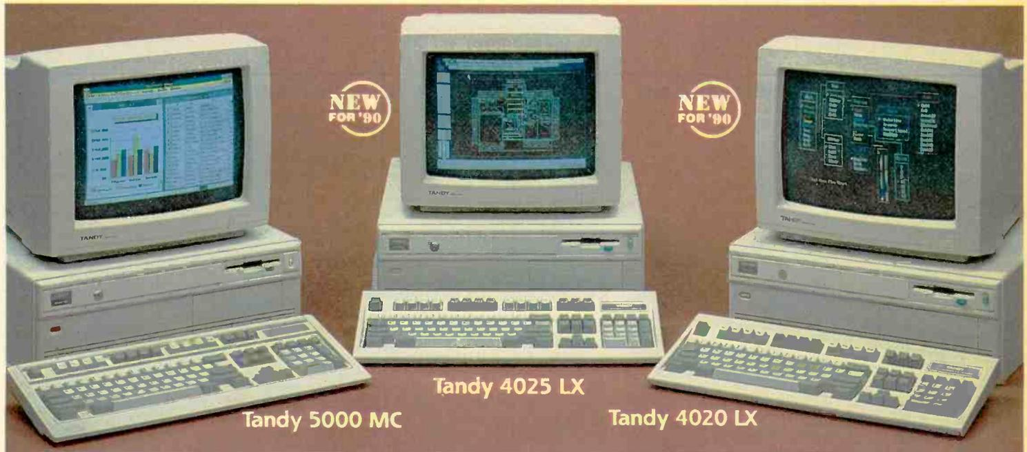
The high-performance answer for power users. IBM® Micro Channel™ compatible architecture provides a fast 32-bit data path. The 5000 MC's Intel® 80386™ microprocessor operates at 20 MHz, and a memory cache controller provides RAM-fast access to your data. 2 MB RAM, VGA graphics built in. UL listed AC. 25-6000\* (TSP available) . . . . 4999.00
