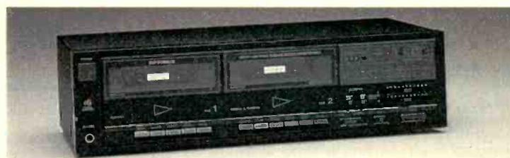
Response:  $\pm 3$  dB: 60-14,000 Hz (metal), 60-13,000 Hz (CrO<sub>2</sub>/Hi-Bias/Type II), 60-12,500 Hz (normal/Type I). **Wow and Flutter:** 0.12% WRMS. S/N: 64 dB Dolby on (ref. 3.0% distortion, "A" weighted, metal tape). **Distortion:** 1.5%. **Record/Play Head:** Permalloy. **Erase Head:** Ferrite. **Size:** 4<sup>9</sup>/<sub>8</sub> x 16<sup>1</sup>/<sub>2</sub> x 7<sup>7</sup>/<sub>8</sub>"
