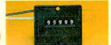
Electromechanical Counter. Extra-rugged device with many uses—at a bargain price! Advances one count with a 12VDC pulse. Counts up to 99,999 with manual pushbutton reset. Easily mounts in a 1<sup>11</sup>/<sub>16</sub> x 1" panel hole. Overall depth: 1<sup>13</sup>/<sub>16</sub>". With leads and data. 277-222 . . . . . 14.95
