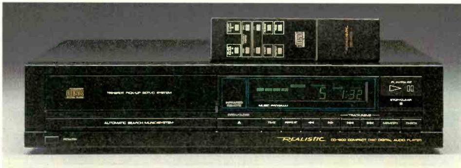
**SPECIFICATIONS.** Frequency Response: 5-20,000 Hz +0.5, -1.0 dB. S/N: 90 dB. Dynamic Range: 90 dB. Harmonic Distortion: 0.05% at 1 kHz. Wow and Flutter: Below measurable limits. Sampling Frequency: 44.1 kHz. Oversampling: 2 times. Signal Processing Rate: 88.2 kHz. Size: 2 3/4 x 14 1/4 x 11 1/2"
