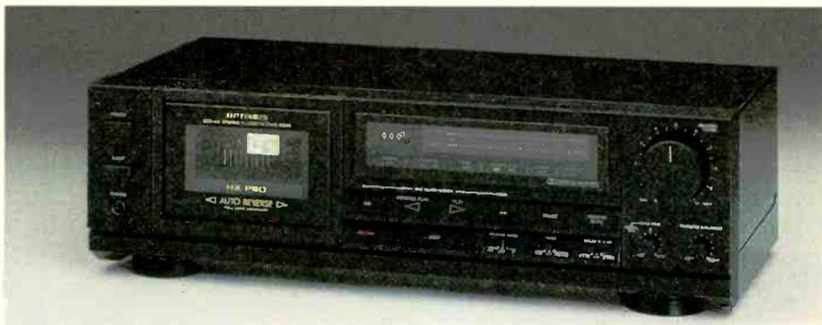
**Response:** ± 3 dB: 20-18,000 Hz (metal), 20-17,000 Hz (CrO<sub>2</sub>/Hi-Bias/Type II), 20-16,000 Hz (normal/Type I). **Wow and Flutter:** 0.065% WRMS. **S/N:** 78 dB Dolby C; 65 dB Dolby B (metal tape). **Distortion:** 1.0% 3rd HD. **Record/Play Head:** Permalloy. **Erase Head:** Double gap ferrite. **Size:** 5 × 17 × 9 1/4"
