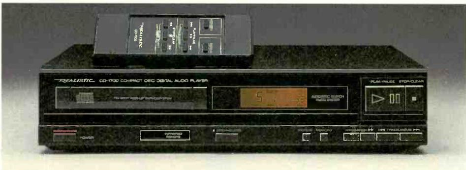
**SPECIFICATIONS.** Frequency Response: 5-20,000 Hz +0.5, -1.0 dB. S/N: 90 dB. Dynamic Range: 90 dB. Harmonic Distortion: 0.05% at 1 kHz. Wow and Flutter: Below measurable limits. Sampling Frequency: 44.1 kHz. Oversampling: 2 times. Signal Processing Rate: 88.2 kHz. Size: 3 x 11 x 13 1/4"
