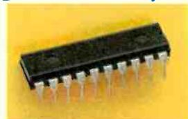
VCP200. Great experimenter's item! This speaker independent LSI device understands seven preset motion and start/stop commands. Clipped audio input—complete system requires few external parts. 20-pin DIP with circuit data. 276-1308 ..... 9.95
