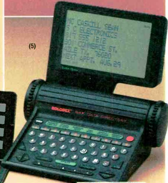
Built-in IR transmitter lets you transfer data between any two compatible Rolodex directories in seconds.
