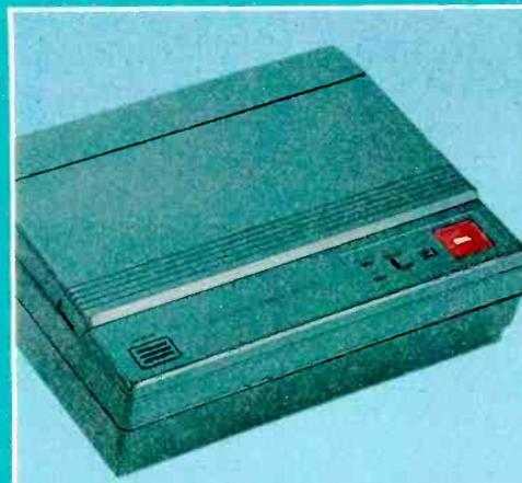
**Security Auto-Dialer.** Triggered by an alarm system or touch of a button. Dials up to three phone numbers, plays message to alert police, fire, physician. Large, easy-to-find "panic" button. For any pulse or tone line. UL listed AC. Backup requires 3 "AA" and 4 "C" batteries. FCC registered. 2<sup>3</sup>/<sub>4</sub> x 9 x 6<sup>3</sup>/<sub>4</sub>". (TSP) 49-433 ..... 99.95
