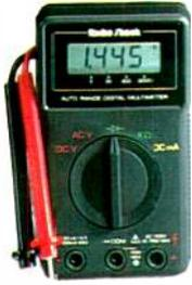
Easy to use! Autopolarity, 5-position control. Select DC volts, AC volts, resistance or DC current—the meter sets correct range automatically. Diode-check lets you quick-test diodes and transistors. Autopolarity protects meter and gives you valid readings if you connect leads to circuit in reverse. Low-battery indicator.  $5 \times 3 \times 1\frac{1}{8}$ ". Requires 2 "AA" batteries. 22-166 ..... 39.99
