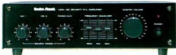
**35-watt public address amplifier with 3-band frequency equalizer**
