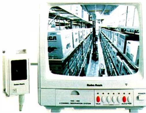
Camera has 6 built-in infrared LEDs that help illuminate dark areas—without visible light.
