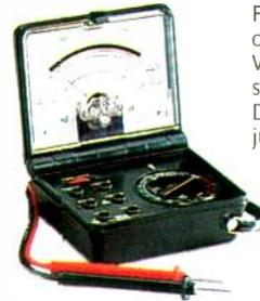
Full-size meter folds for travel or storage. Ideal for tool box. When shut, the movement is shunt-protected from shocks. Detented hinge lets you adjust display angle for easier viewing. 25 ranges. DC and AC volts, DC current, resistance and dB. 20,000  $\Omega$ /volt.  $7\frac{5}{16} \times 4\frac{3}{8} \times 1\frac{5}{16}$ ". open. Req. "AA" batt. 22-211, 34.99
