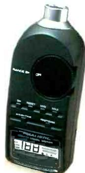
Provides precise readings when setting up stereo or PA system. Reads 60 to 120 dB SPL, and has "A" or "C" weightings. Carry case. **32-2055 . . . 59.99**
