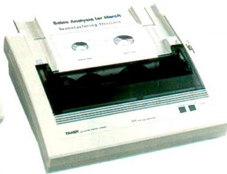
**DMP 203.** Prints up to 240 characters per second and contains four resident fonts. Has 24-pin print head for high-resolution printing. IBM Proprinter X24/24e emulation. Has automatic paper loading, push tractor for fanfold paper, friction-feed for single-sheet use. Only 7.9 lbs. 4<sup>3</sup>/<sub>4</sub> × 15<sup>3</sup>/<sub>8</sub> × 11<sup>3</sup>/<sub>8</sub>". (TSP)
