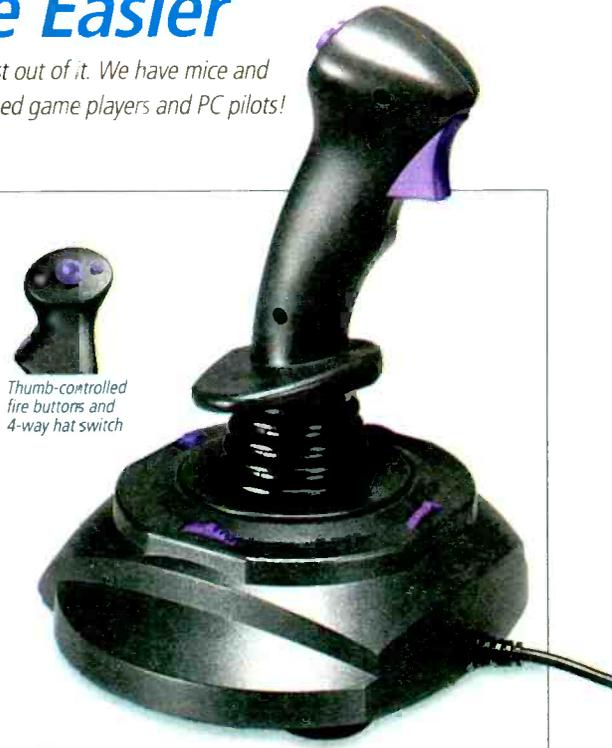
Thumb-controlled fire buttons and 4-way hat switch
