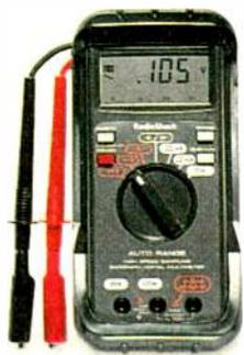
**Edge-placed controls for easy one-hand mode/range selection**
