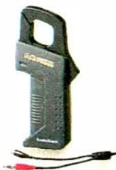
Use with air conditioners, refrigerators, space heaters—any AC appliance. Just clamp probe around the current carrying wire and read the result on your multimeter. With banana plug test leads for connection to most multimeters. Measures up to 300 amps. **22-601** . . . . . **29.99**
