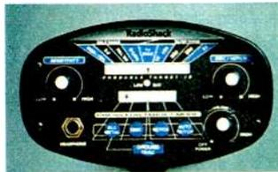
Readouts indicate the metal type.
