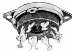
**No. 540-1-E**—A socket of standard high dielectric black bakelite for mounting with crimped mounting saddle and employing in standard applications spring brass alloy. Contacts, cadmium plated. The contact design in this socket is of the wrap-around type and the solder lug illustrated is of spade design.
