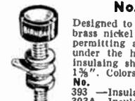
Designed to leave no metal part exposed on the panel. The 3/8-24 brass nickel plated sleeve has a 10-32 threaded hole at the end permitting a connection at the end of the jack or to the lug under the head. Either assembly available complete with nut, insulating shoulder washer, lock-washer and lug. Length overall 1 3/4". Colors: red or black.
