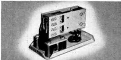
*Rubber shock mount for high-power vibrators. Low-power vibrators are mounted in the conventional rubber sock.*
