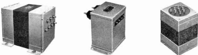
By using the new design of heavy steel end-bells, both mechanical strength and eye appeal have been added together with other features such as more effective shielding, better insulation, etc. Durable ceramic terminals are mounted on steel end panel to assure adequate insulation. End bells are filled with rubber-seal compound.
