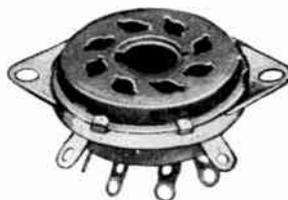
No. 535L-1-E—Is identical in design with the 535-1-E socket. Both sockets employ the same type of mounting and contact designs. The 535-1-E employs low-loss mica-filled bakelite for insulation for use in appropriate circuits. For such application the customary plating provided on contacts is silver. The crimped-on mounting saddle illustrated indicates ground lugs which may be provided for convenient chassis grounding.
