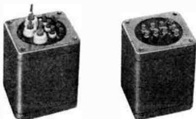
All Thermador filament transformers have center-taps. They are designed to provide accurate voltage output at rated leads with good regulation, and are insulated to stand well over twice the peak working voltage plus one thousand volts.
