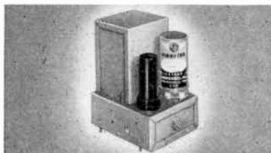
**601** A typical standard vibrator converter for power pack use. Input: 6 volts DC; Output: 300 volts DC; Output power: 30 watts; Dimensions: 4 $\frac{1}{4}$ " x 4" x 6"; Weight: 6 pounds.
