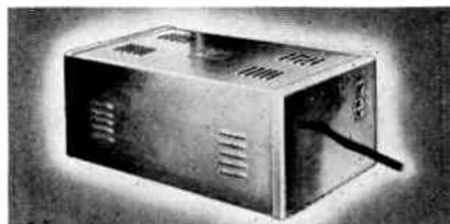
**146** A standard E-L vibrator inverter operating on 32 volts DC for powering radio receivers and transmitters, coin phonographs and other equipment which demands 350 watts power. Input: 32 volts DC; Output: 115 volts AC; Output power: 350 watts; Dimensions:  $16$ " x  $10$ " x  $8\frac{3}{8}$ "; Weight: 48 pounds.
