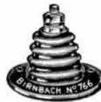
Base measures 2" dia. with 3 holes on a 1 1/8" circle, for No. 6 screws. Supplied complete with 12-24 nickel-plated brass screw and nuts. The No. 766J has a No. 403 Jack. Available white or brown glaze.
