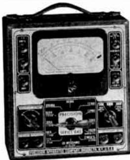
Series 845 is a reliable, highly accurate, multi-range tester of moderate sensitivity for more accurate measurements in sensitive communications and electronic apparatus. Its dual-sensitivity feature, suits Series 845 to the requirements of laboratory, maintenance and production testing.
