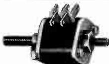
Coprox Model CX-4D4F23, a full wave rectifier with high conversion efficiency, for electronic control work. Rated at 5 volts A.C., 40 milliamperes D.C. continuous. Fully enclosed. Mounts on a single screw.
