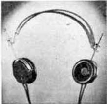
For use where HIGH FIDELITY and extended frequency response are of paramount importance. (60 to 10,000 cps. Corrected for rising response below 200 cps.) Especially suited to monitoring, sound measurement, audiometry, and similar exacting headphone applications. Sensitivity approx. 1.5 bars per volt at 1,000 cps. Impedance over 80,000 ohm. at any frequency.
