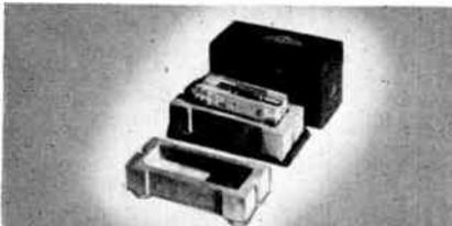
*Sponge rubber envelope mounting which cushions the high-power vibrator against shock. This mounting and the rubber shock mounts are used in the plug-in rectangular container.*
