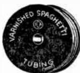
A flexible tubing, heavily varnished, in attractive colors. Average dielectric strength, 5000 volts. Will accommodate from No. 10 to No. 18 wires. Furnished in one length —20 feet long on handy spools.
