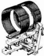
A small, unusually compact, highly efficient Assembly designed for direct mounting on condenser. Ideal for low powered transmitters and exciter stages or in conjunction with B & W Type BL coils in interstage coupling. Six interchangeable plug-in coils provide a complete range, from 5 to 160 meters.
