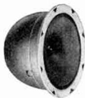
As used in 15" coaxials. Designed to reproduce the high frequencies from 4,000 to 15,000 cps., when used with dividing network (such as A40-1) and suitable low frequency speaker. Impedance, 16 ohms. Overall diameter, 5 1/2". Depth, 3 5/8". P.M. design.
