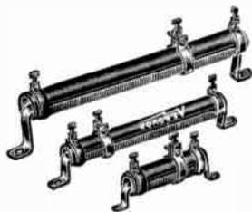
Adjustable resistors combining adjustment to any resistance value within unit's range, with positive, permanent, non-fluctuating qualities of wire-wound resistor. Each Slideohm Resistor is provided with horizontal mounting brackets and one adjustable contact slider.
