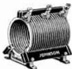
Wound with plated edgewise copper strip and supported by low-loss hard rubber insulation, these inductors present a very commercial appearance and safely handle up to 1000 watts. Sizes for all bands and for impedance matching networks. Also available on special order with Mycalex or Bakelite insulation. Other edgewise wound inductors are listed in the Commercial Catalog.
