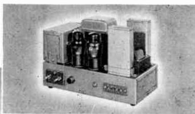
**618** A standard E-L vibrator converter with tapped output for transmitter application. Input: 12 volts DC; Output: 600 volts DC; Output power: 200 watts; Dimensions: 11 $\frac{1}{4}$ " x 6 $\frac{1}{4}$ " x 7 $\frac{1}{16}$ "; Weight: 25 $\frac{1}{2}$  lbs.
