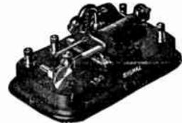
The commercial relay is well designed and constructed for long, continuous service on commercial lines. Heel iron and armature are made of Norway iron. Has rubber covered adjustable coils. Mounted on mahogany finished wood sub base and cast iron black enamel base.
