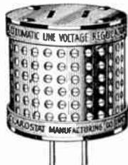
Designed for use with 110-volt socket power radio sets not equipped for line ballasts. At 110 volts, the resistance of the units is low and the voltage drop across them is negligible. As the line voltage increases, however, the resistance of the units increases with a consequent increase in voltage drop across
