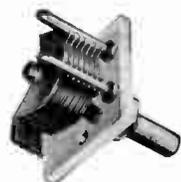
For tuning or trimming on high frequencies. Cadmium plated soldered brass plates. Isolantite. Base mounting, single hole panel mount, or panel mounting with bushings. 140 mmf. size 1 1/2" high x 1 1/2" behind panel.
