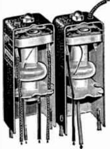
Supplied in matched pairs; designed to provide a low-impedance link-coupled filter circuit for superhet receivers. Input unit has tuned primary and low-impedance secondary; output unit has low-impedance primary and tuned, high-impedance secondary. Coupling is set to give optimum gain; selectivity provided by crystal in link circuit. In black crackle cans.
