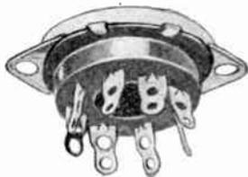
No. 535-1-EN—This type socket is identical with the 535-1-E socket shown except that it employs the crimped mounting saddle inverted so that it may be mounted on the top of the chassis for greatest economy of space in the wiring area underneath. It can be specified with either high dielectric black bakelite or mica-filled low-loss bakelite with either wrap-around or cutting-edge type contacts.
