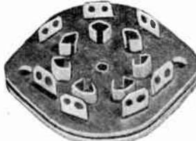
**No. 43-1-D**—Standard type 43-1-D socket employing cutting-edge contacts of spring alloy brass, cadmium plated. Bottom and top plates are  $\frac{3}{64}$ ", laminated insulation, XX specifications.
