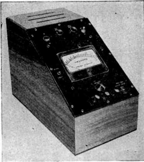
For high-speed testing of capacitor leakage resistance, insulation resistance and insulation measurements in production and inspection of components. Extra charging terminals charge capacitors prior to test. Broad scale meter dial with wider than usual spacing at high end of scale.
