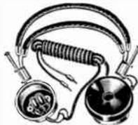
A fine headset of bi-polar construction having a laminated magnet structure of the best grade chrome steel; shell of polished aluminum; molded cap; adjustable fabric-covered wire headband; high-grade tinsel cords with terminals entirely enclosed. A truly great phone combining features not before incorporated in a low cost headset. Extreme sensitivity to weak signals is attained.
