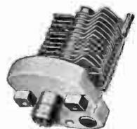
For S.W. and ultra-S.W. For I.F. tuning, trimming R.F. coils or gang condensers, general padding, etc. Constant capacity under any conditions of temperature or vibration. Size 100 mmf.  $1\text{-}\frac{7}{32}$ " x  $15\text{-}\frac{1}{16}$ " x  $1\text{-}\frac{7}{32}$ ". Isolantite base. Cadmium plated soldered brass plates.
