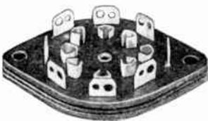
No. 43-1E-3—Laminated socket employing three insulating plates with adjacent contacts alternated above and below the center plate. This special construction provides a 50% increase in normal between-contact voltage breakdown. National Fabricated Products produced this particular design for high voltage applications in rectifier and amplifier circuits. Insulation may be specified in X, XX, or XXX bakelite and wax impregnated where high humidity operating conditions are contemplated.
