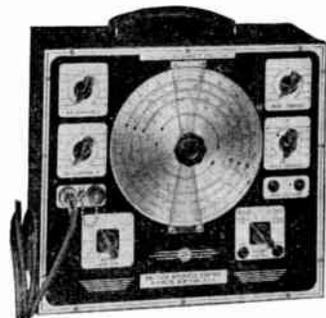
● Six Bands: 90 KC to 88 MC. ● Accuracy—Constancy of calibration: MAXIMUM of 1% DEVIATION on all bands, insured by use of the "PRECISION" developed "UNIT OSCILLATOR" construction. ENTIRE "UNIT OSCILLATOR" is SINGLE-POINT-MOUNTED, providing positive freedom from effects of mechanical shock, eliminating the need of costly, useless, single frequency reference crystals.
