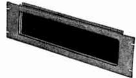
These panels are made so that the meters may be recessed from the front of the panel. Meters are protected by a plate glass insert, allowing 3/4" clearance in back of panel. A blank bakelite sub-panel is provided. The clear sub-panel space is 4½"x15" on the 19" wide panel which is sufficient for 4-3" meters. On the 24" and 30" wide panel the clear sub-panel space is 5¼"x20" and 5¼"x26" respectively.
