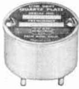
**TYPE C & S CRYSTAL**— $1\frac{1}{2}$ " dia.,  $\frac{3}{8}$ " high (exclusive of pins), Standard 0.125" pins on  $\frac{3}{4}$ " centers. Standard tolerance 0.01%, 4 cycles/Mc/°C. (2 cycles/Mc/°C or less drift slightly higher in price).
