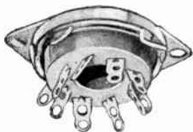
No. 535L-1-EG — The socket illustrated above is identical with the 535L-1-E shown below with the exception of the crimped-on mounting saddle providing ground lugs which are available. Crimped-on mounting saddles may be specified with one to four ground lugs to provide convenient grounding points to the chassis.
