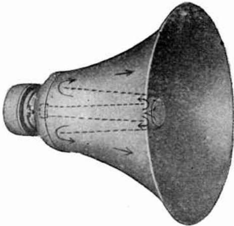
ALL RACON RE-ENTRANT SPEAKERS have base and inside tone arm made of aluminum castings, outside bell of heavy gauge aluminum spinning, and center reflecting section of RACON ACOUSTIC material to prevent resonant effects prevalent in all metal reflecting surfaces. Sturdy construction makes them practically abuse-proof.
