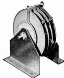
Use the Selcocharger as an "A" eliminator. Maximum AC input 18 volts, single phase. DC output 12 volts, 4.5 amperes DC into a resistive or inductive load.
