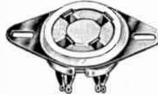
**STEATITE SOCKETS** — Recommended for high frequency work where high temperatures are encountered such as in transmitters, amplifiers having high output and for extensive replacement service use. Plates have slotted mounting holes to fit riveting centers from 1 1/2" to 1 3/4".
