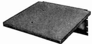
These standard tables are rigidly made of 1/8" thick furniture steel. The rounded front corners are of seamless construction and the flanges of the shelf are folded in to provide smooth edges underneath. They are securely mounted to regular 1/4" steel panels, size 10½"x19". They may be obtained in two sizes and finishes as listed below. The tables are 22" wide to give full working space across the front of the racks when mounted in place. Shipping weight is 35 lbs.
