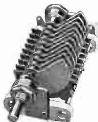
Exceptional unit for ultra-s.w. receivers and transmitters particularly compact transmitters. Plate spacing—.0715". Great for tuning crystal controlled transmitter amplifier stages or for neutralizers up to 1000 volts. In midline (MX) and straight line cap. types (SX).
