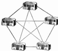
The Model CS-1010 "Super Chief" is made up exclusively of master stations. Any number up to ten may be had in the system. This system permits five two-way conversations to be held simultaneously without interference or
