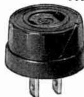
Filternoys Diverter F18 is a compact 0.1 mfd capacitor in a conveniently small bakelite plug-in coupler for use across domestic power lines in which the neutral wire is grounded. The capacitor diverts interference from the high potential side of the power line to the grounded neutral side. Use on floor or table lamps, cigarette lighters, and the radio.
