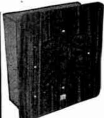
**Model 90-WS—An ideal speaker for auditoriums, cafeterias, offices, or other locations where a neat, attractively housed, wall-mounted unit is preferred. It contains a 12-inch, high fidelity, permanent magnet speaker with line matching transformer. It is capable of handling up to 10 watts of power with high fidelity reproduction. Its beautifully finished walnut-housing measures overall 19 5/8" x 17 7/8" x 8 1/2". Cat. No. U-1035.**
