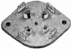
**No. 43-1-A** — Standard type socket with cutting-edge contacts of spring alloy brass, cadmium plated. Top plate  $\frac{3}{64}$ " laminated insulation, XX specifications. Bottom plate  $\frac{3}{64}$ ", linen base laminated insulation, XX specifications.
