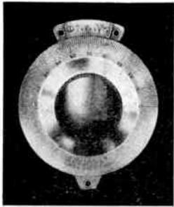
The four-inch N Dial has an engine divided scale and vernier. The vernier is flush with the scale. The planetary drive has a ratio of 5 to 1, and is contained within the body of the dial. 2, 3, 4 or 5 scale. Fits 1/4" shaft. **Specify scale.**
