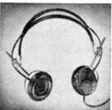
Developed for COMMUNICATIONS work where light weight, durability, and uniform response are required. Soft rubber housing insures good ear seal and wearing comfort over long hours of constant use. High output impedance .008 mfd. (40,000 ohms at 500 cps), response 100 to 10,000 cps.
