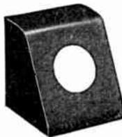
These meter cases may be obtained for 2" and 3" meters. Substantially made from steel, with welded joints, and finished in black ripple enamel. Top front corner is rounded to harmonize with "streamlined equipment." Size is 4½" x 4" x 4".
