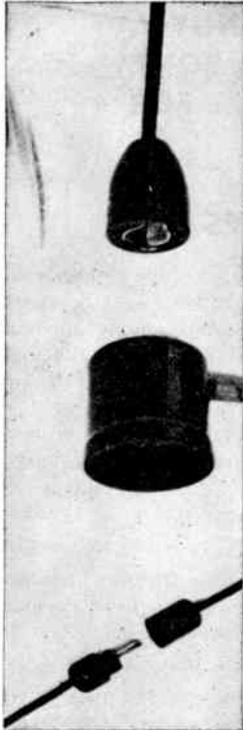
Used especially for transmitter tubes operating at high temperatures. Molding can be unscrewed for inspection. Wire clamped in annular ring eliminates need for solder.
