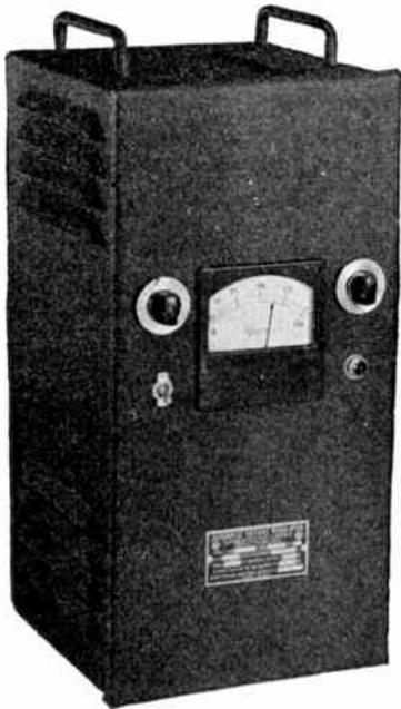
The SECO automatic voltage regulator maintains a constant output voltage with variations in input voltage or output load current. This regulator consists of a special bridge and thyatron tube circuit which detects any variation in a c line voltage and authorizes a Motor-driven POWERSTAT Variable Transformer to correct for a constant output voltage.
