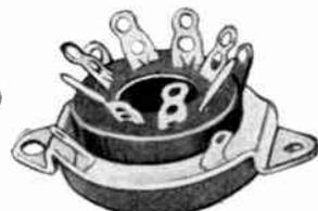
No. 35-1-E—The 35-1-E socket is identical with the 530-1-E in type of insulation, contacts available, and contact lugs available. The 35-1-E socket is mounted with the pressed-on mounting plate and may be obtained with four standard mounting centers— $1\frac{1}{2}$ ",  $1\frac{11}{16}$ ",  $1\frac{3}{4}$ " and  $1\frac{7}{32}$ ". Two variations in mounting centers are illustrated.
