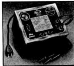
A valuable accessory where an older type capacitor analyzer is already in use. Incorporates the Quick-Check dynamic testing feature for detecting opens, shorts, intermittents, r.f. impedance and power factor—with capacitor in or out of circuit. Capacitance bridge and leakage test not included. Size, 5" x 6" x 4 1/2" high. Weight, 5 1/2 lbs.
