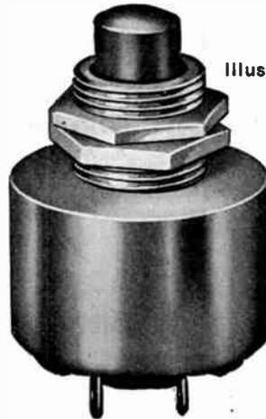
A new push-button type switch with a double break shorting bar feature for panel mounting applications.  $\frac{3}{8}$ " diam. Cadmium plated brass case with a sturdy threaded sleeve  $\frac{1}{2}$ -32. Normally open and normally closed circuits. Rating is 15 amps. at 115 volts A.C.
