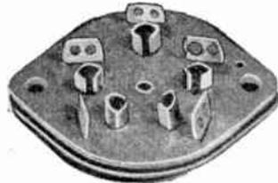
**No. 43-1-B** — Standard type socket with cutting-edge contacts of spring alloy brass, cadmium plated. Bottom and top plates  $\frac{3}{64}$ ", laminated insulation of XX specifications.
