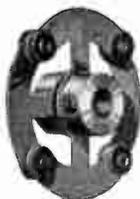
The sides of coupling are insulated from each other, allowing instruments in gang to be operated as independent electrical units. Bakelized canvas with brass bushings for  $\frac{1}{4}$ " shaft. Four rust proofed and hardened steel set screws provide against shaft slipping. Overall diameter  $1\frac{1}{2}$ ".
