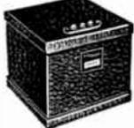
Designed especially to fit into the Signal Spotter but may be used with any Crystal Oscillator unit! Holds up to four mounted crystals; provides accurate temperature regulation within plus or minus 1 degree C. Steel outer shield is 4 3/4" square by 4 3/4" high; crystals in inner chamber of heavy cast aluminum with thick insulating material in walls; terminals on top for connection of 6.3-volt heater supply.
