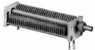
**K-150-050**—One of the most popular "specials" because of the high capacity available for the small panel space required. Maximum capacity of type illustrated 150 mmf., spacing .050". Available in other capacities and plate spacings, and with special mounting brackets to your specification. Other special types available with dual or even up to five sections.
