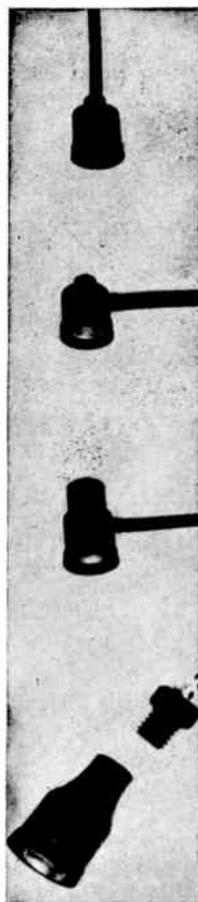
Lead brought through insulating pocket on top. Lead, eyelet and clip soldered together.
