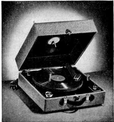
Model No. 101 phonograph unit is a record playing device for either ten or twelve inch phonograph records and it comprises a 78 R.P.M., rim drive phonograph motor with a ten inch flock covered turntable. The phonograph pickup is of the off-set arm type with a crystal cartridge. Output for 500,000 ohm load.
