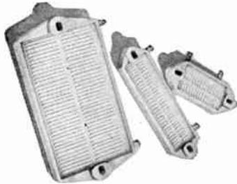
Vitrohm Plaque Resistors are flat in form. The resistance wire is arranged on a rectangular ceramic base to give the lowest obtainable values of inductance and distributed capacitance. Inductance at frequencies up to 1000 kilocycles and distributed capacitance up to 5 megacycles are so low in value that they are negligible.
