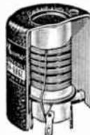
Standard type air-core coils of superior construction, designed to cover the broadcast band from 545 to 1580 kc (190 to 550 meters) with a 365-mmfd tuning condenser. Excellent for replacement use and are used as original parts by discriminating set-builders and experimenters in the design and construction of broadcast band receivers. All coils have high-impedance primaries, wound with Litz wire, fully protected against humidity. Shields are 1 1/2" x 2 1/2".
