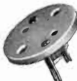
The "XS-2" is a special crystal socket designed to conserve space and provide a low loss mounting for standard crystal holders. Made with heavy-duty spring contacts and mounted on glazed Isolantite. Can also be mounted inside "SWF" coil forms for changing coil and crystal in one operation. Overall diameter  $1\frac{1}{16}$ ".
