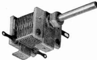
**K-100-2B**—A very popular "special" with mounting brackets and shaft length to specification. Maximum capacity 100mmf. Plate spacing .022". Available in other capacities and plate spacings.
