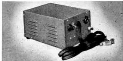
**502** A typical E-L standard vibrator inverter operating on 12 volts DC for powering radio receivers and electric appliances. Input: 12 volts DC; Output: 115 volts AC; Output power: 100 watts; Dimensions:  $9\frac{3}{8}$ " x  $6\frac{3}{8}$ " x  $4\frac{7}{8}$ "; Weight:  $14\frac{1}{2}$  pounds.
