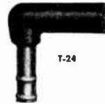
Code T-24 Distributor Suppressor — Is an angle type with screw in cable. The spring brass insert has two rolled bosses, one to hold suppressor rigid and the other to snap into the groove of the distributor well.
