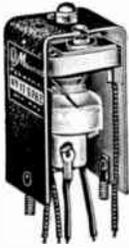
Special, close-coupled transformers for use in "Lamb" type noise-silencer circuits. Complete range of I-F frequencies available, with air or mica dielectric trimmers; air-tuned units are 2" sq. x 4 1/2"; mica-tuned units 1 1/2" sq. x 3 1/2".
