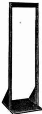
Where a sturdy mounting for a number of panel and chassis units such as in a transmitter, public address system, etc., is desired, allowing complete accessibility to all parts, this line of Relay Racks is indispensable. The one-eighth inch steel channels, three inches deep, are held together by angle cross-pieces of the same material. The base design has been improved to incorporate a chassis-type bottom, together with the usual side angles, making the rack stronger and more stable.
