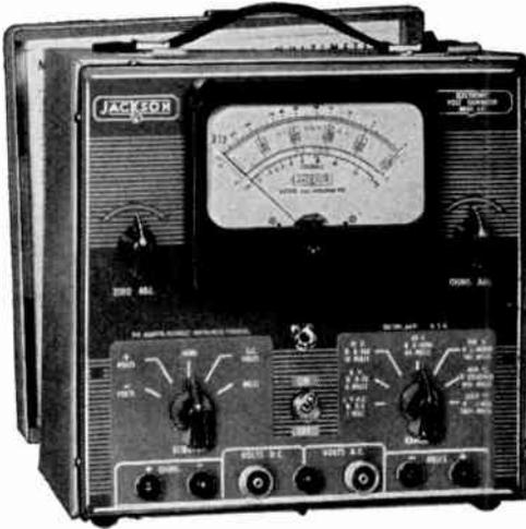
BOTH A.C. AND D.C. VOLT RANGES ARE ELECTRONIC. This provides the maximum of sensitivity and overload protection for all A.C. ranges as well as D.C. and ohms ranges.
