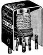
Entirely new design. Specially built for compact I. F., Super-Het and Auto Radio receivers. Wound on  $\frac{1}{2}$ " bakelite form. Four bank windings with Litz wire. High impedance primaries. Shield cans  $1\frac{3}{8}$ " x  $1\frac{3}{8}$ " x  $\frac{1}{2}$ ". Spade bolt mountings. Cover 190 to 450 meters with 365 mmf. condenser.
