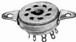
No. 35L-1-E—The 35L-1-E socket illustrated employs mica-filled low-loss insulation and may be specified with either the wrap-around or cutting-edge type contact. It is shown with pressed-on mounting plate which is available in  $1\frac{1}{2}$ ",  $1\frac{11}{16}$ ",  $1\frac{3}{4}$ " and  $1\frac{7}{32}$ " mounting centers.
