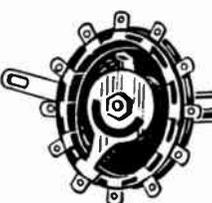
Positive snap action — strong wiping contact grounded to shaft and bushing. In operation contact breaks between makes.
