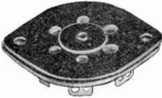
**No. 43-1-C** — Standard type 43-1-C socket employing cutting-edge contacts of cadmium plated spring alloy brass. Bottom and top plates  $\frac{3}{64}$ ", laminated insulation of XX specifications.
