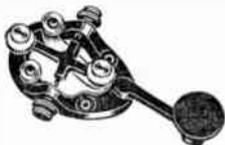
A sending key with molded phenolic base. Key lever is heavy phosphor bronze. Spring steel lever spring. All hardware finely machined brass. With stands voltage breakdown between contacts of 1000 volts raw A.C. and insulation of 1000 megohms.
