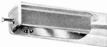
Many tens of thousands of Shure Magnetic Cutters are in use throughout the world in Home Recording Sets. These cutters operate directly from the voice coil winding of the output transformer. A stiff moving element permits recording on practically all recording materials. Furnished with 36" flexible lead. Overall length 3 3/8". Shpg. wt. 8 oz.
