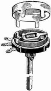
A dependable wire wound control of uniform resistance change for power requirements up to 2 watts. Tight, uniform windings assure utmost accuracy. Spiral Spring Connector between rotor arm and center terminal eliminates noise. Diameter  $1\frac{1}{4}$ " ; depth behind panel  $\frac{3}{16}$ " ; shaft length  $2\frac{1}{8}$ " from control face. Illustration shows cover removed, although covers are supplied with controls. Includes new IRC Control Tag.
