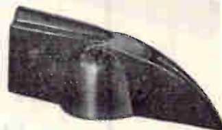
No. 2350 Zephyr bar knob Length 2". Height 5/8". 1/4" molded hole, metal insert set screw mounting.
