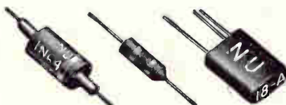
Actual size illustrations. Left to right, point-contact diode, "Union" diode, transistor.
