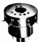
G-C DUD-DECAL TV TUBE TEST SOCKET ADAPTER —Designed for making measurements of voltage, resistance and video from the base of the picture tube. It is inserted between C.R. tube base and its socket. Cat. No. 9251 Net $1.95
