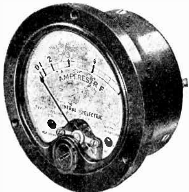
Type DW-52 ammeter in a molded Textolite case
