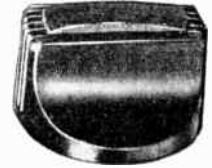
Cat. No. S-453-1 Walnut and black. No brass insert. Molded hole to fit standard \frac{1}{4} " shaft with one set screw. Diam. 1", ht. \frac{39}{32} "
