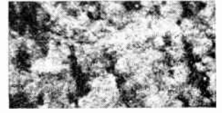
Particular attention is invited to the absence of "clusters" of particles. Above is a photomicrograph of competitive tape enlarged 50 X.
