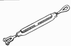
HEAVY DUTY TURNBUCKLE TW-12 Made from forged steel, galvanized to prevent rust. Jaw and eye type 1/2" x 6".
