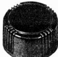
Cat. No. S-451-7AA Black, walnut, ivory. Molded spring type shaft hole fits standard \frac{1}{4} " shaft with one set screw. Diam. \frac{13}{16} ", ht. \frac{39}{32} "
