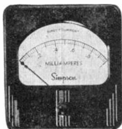
MODELS 27, 37, 47, 57 3 1/2" RECTANGULAR CASE. Width, 3"; height, 3 1/8". Mounts in round hole. Body diameter, 2 3/4". Scale length 2 9/16". Bakelite case.
