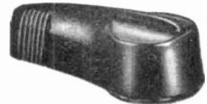
No. 2110 Lgth—overall 1 5/8". Hght. 1 7/32". Dia. 3/4". 1/4" molded hole, metal insert, knurled hole mounting.
