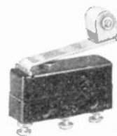
MODEL Z Roller Leaf Actuator ZLD-0033 O.F. 2 OZ. MAX. 5 AMPS 120-240 V.A.C.
