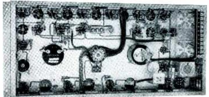
*Inside view of complete modulator unit with back cover removed. The extreme simplicity of the Cascade Phase Shift circuit is well illustrated.*
