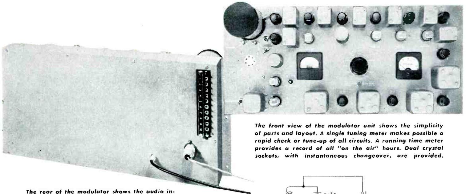
The rear of the modulator shows the audio input and RF output receptacles and the interconnecting terminal strip.
