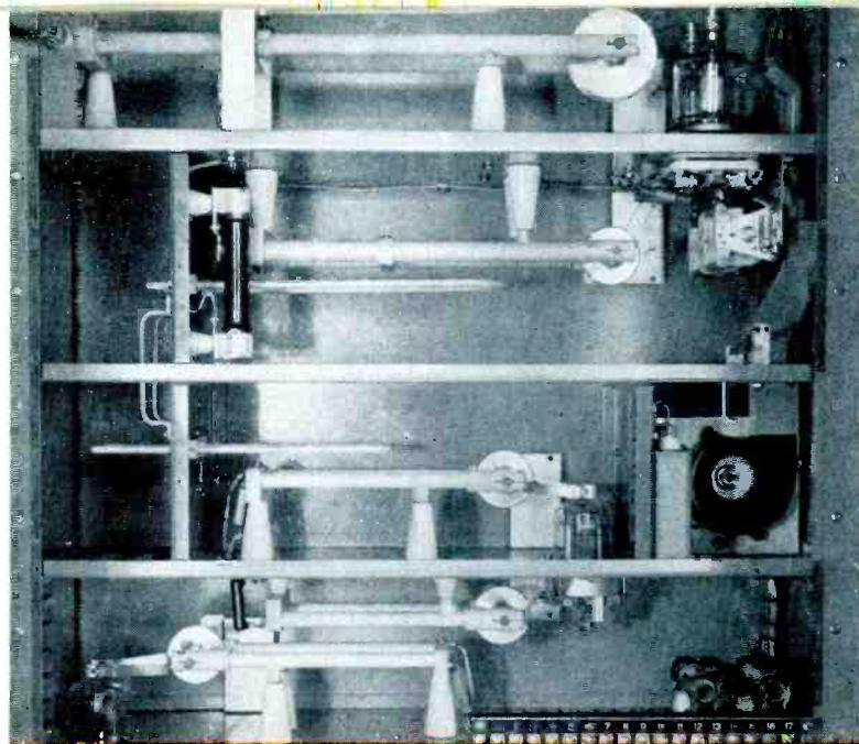
*The view above shows the linear type tank circuits used on all stages operating above 30 MC. Though more expensive than the conventional "coil and condenser" type the use of linear tanks assures stability, reliability, high efficiency, high spurious signal attenuation and ease of adjustment.*
