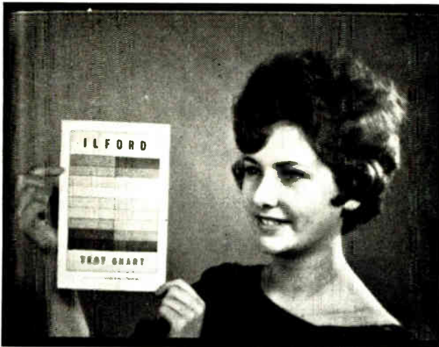
Fig. 4. Picture of model taken with a television camera using an image orthicon with a BiAg photocathode.
