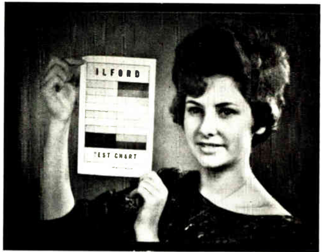
Fig. 5. Picture of model taken with tri-alkali image orthicon used in the camera.
