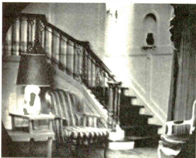
Fig. 8. A picture taken from a color monitor using the RGB system with green tube of camera mis-registered.
