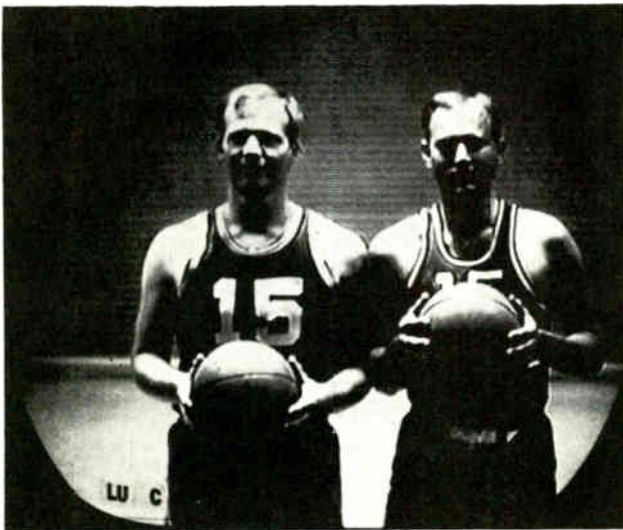
Fig. 12. A photograph of the monitor with lighting in the scene coming from overhead discharge sources alone. This simulates a sideline position of players with no lighting equipment located ahead of the subjects. The ratio of horizontal to vertical surface illumination is about 10:1.
