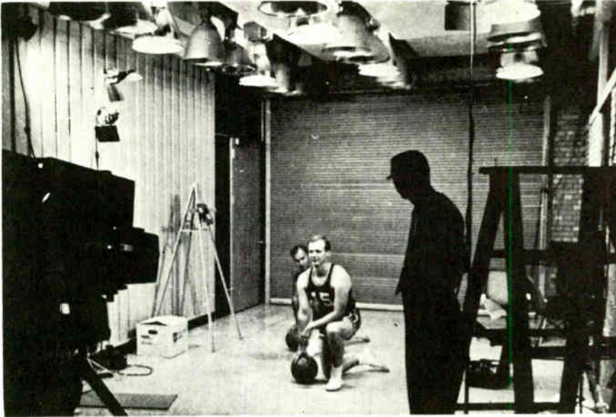
Fig. 11. An overall view of the test site. Discharge sources were used in overhead industrial-type lighting equipment, with supplementary lighting from portable tungsten-halogen units seen at upper left.
