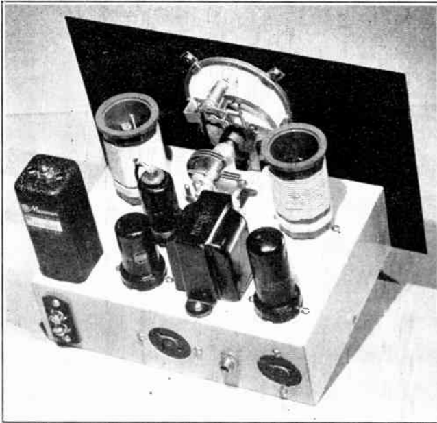
FIGURE 26. REAR VIEW OF THE RECEIVER. The detector coil is to the left, directly above the detector tuning condenser, and the oscillator coil is to the right. Antenna terminals, power socket, speaker plug socket, and earphone jack may be seen on the back of the chassis.
