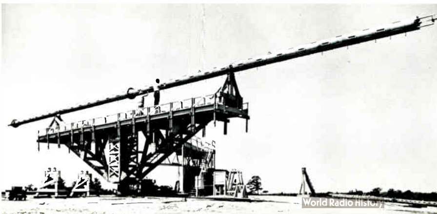
This photo shows an RCA Ultragain Antenna being pattern tested on the 15 ton turntable at the Gibbsboro, N. J. antenna test site.
