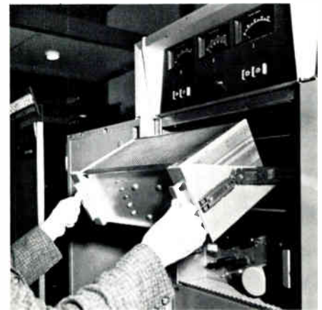
Chassis units slide forward on rails for easy inspection.
