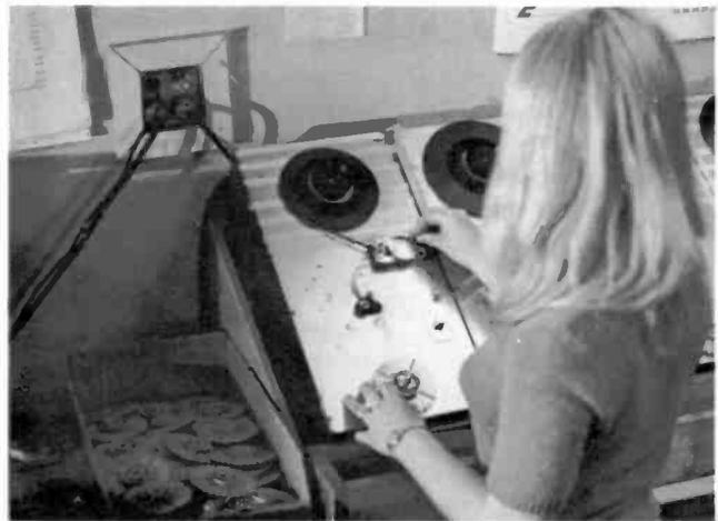
*Cleaned spools are reloaded with fine lubricated tape to customer's exact timing order, then completed cartridge is tape spliced and reassembled before final inspection, testing and packing.*
