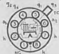
Note.—Type 6K8GT has Pin 1 connected to metal shell.
