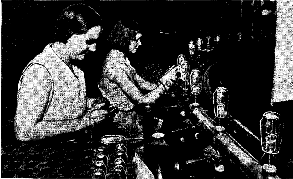
One of the giant semi-automatic pumping machines on which the valves are exhausted to a high degree of vacuum.
