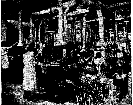
One of the giant semi-automatic pumping machines on which the valves are exhausted to a high degree of vacuum.
