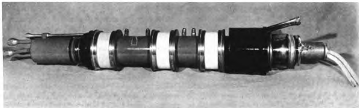
Fig. 6—The Eimac 5-kw uhf klystron for TV.
