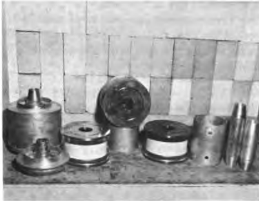
Fig. 7—Tube cavity parts and drift tube sections.
