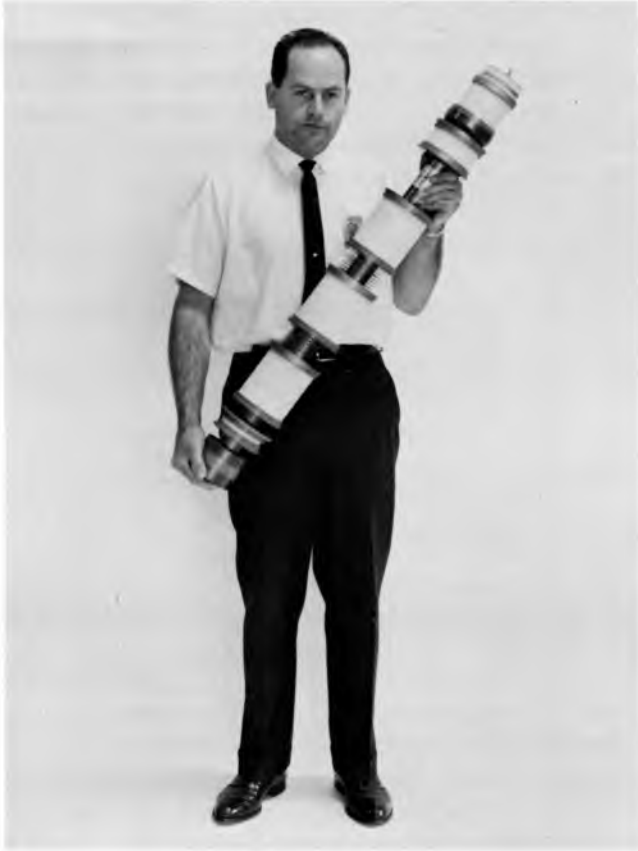
Figure 11—Recommended Method of Hand Carrying Eimac Klystrons.
