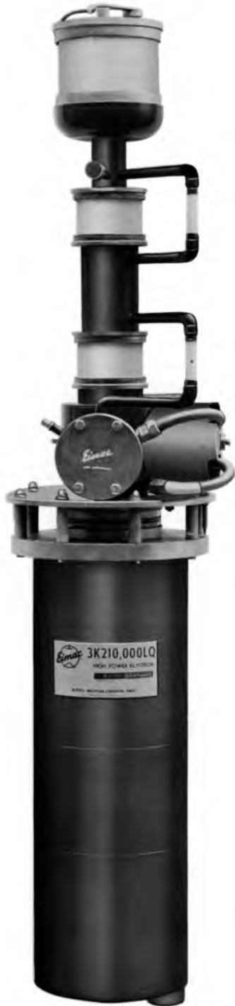
Eimac 3K210,000LQ. This 75 kW klystron is used in many tropo-scatter systems spanning distances up to 440 miles. This klystron is unique in that its input and penultimate cavities are external but its output cavity is integral.
