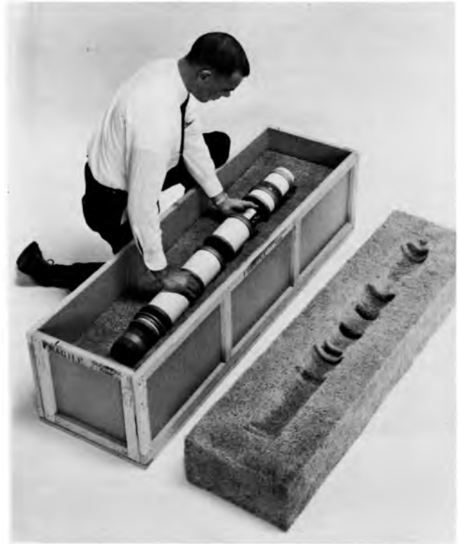
Figure 10—Storage of Klystron in Shipping Crate.
