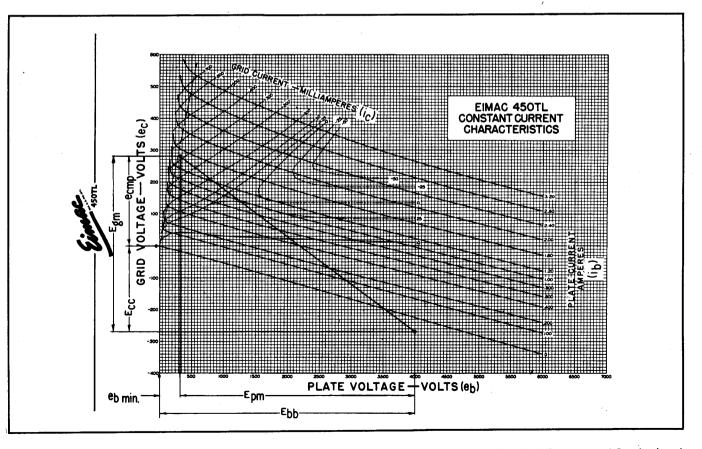
Figure 3. Method of determining  $e_{cmp}$  and  $i_c$  on 450TL constant-current characteristics from values of  $e_{bm1n}$  and  $E_{pm}$  found in steps 6 and 7 and value of  $i_{b}$  found in step 10. The value of  $E_{cc}$  and  $E_{gm}$  from steps 13 and 14 and the operating line are also shown.
