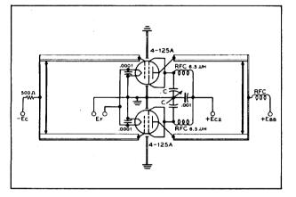
Screen-tuning neutralization circuit for use above 100 Mc. C is a small split-stator capacitor.  $C(_{uufd}) = \frac{640,000}{f^2 (Mc.)}$ , approx.
