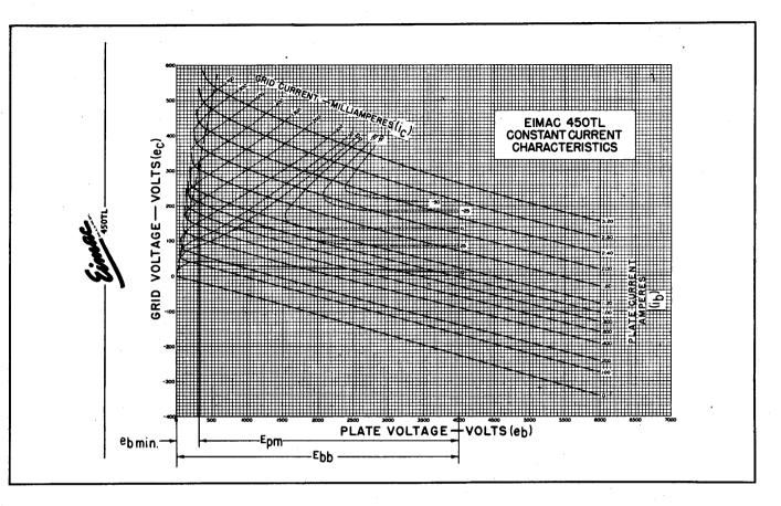
Figure 2. 450TL constant-current characteristics showing method of determining  $e_{bm1n}$  and  $E_{pm}$  in steps 6 and 7 from value of  $i_b$  obtained in step 5.
