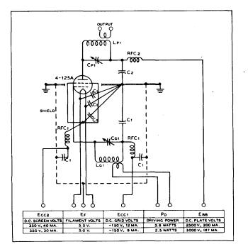
Typical radio-frequency power amplifier circuit, Class-C telegraphy, 500 wátts input.
