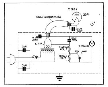
Figure 1. Peak vacuum tube voltmeter for making  $E_{\rm gm}$  or  $e_{\rm cmp}$  measurements.
