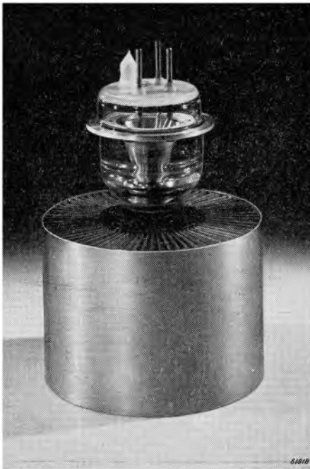
Fig. 11. Triode TBL 6/6000 with air-cooled anode. A cooling jacket with baffles is brazed to the anode and the air passes upwards through the baffles. Anode voltage 6 kV. R.F. output 6 kW. Anode dissipation 5 kW.
