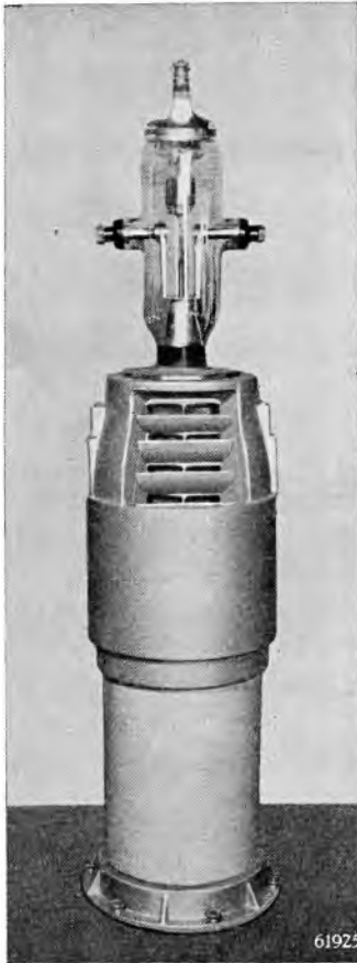
Fig. 8. Triode TAL 12/20 in an air distributor. The air is applied from below, is then separated into numerous horizontal ducts, one above the other, and passes along the anode, leaving the distributor by way of similar ducts, of which the outlets are partly visible in the figure.
