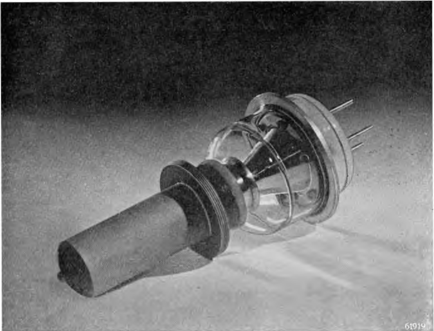
Fig. 3. Triode with thoriated tungsten heater: TBW 6/6000. The anode is water-cooled.
