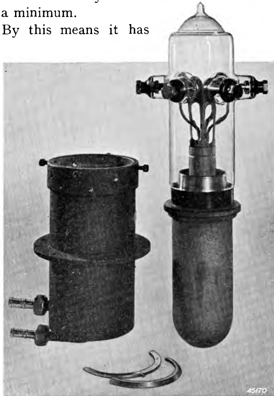
Fig. 9. Sketch of the water jacket for the valve TBW 12/100. The copper spiral winding for increasing the turbulence of the cooling is shown, and in the separate circle the automatic waterseal which enables a quick change-over to new tubes, is depicted.
