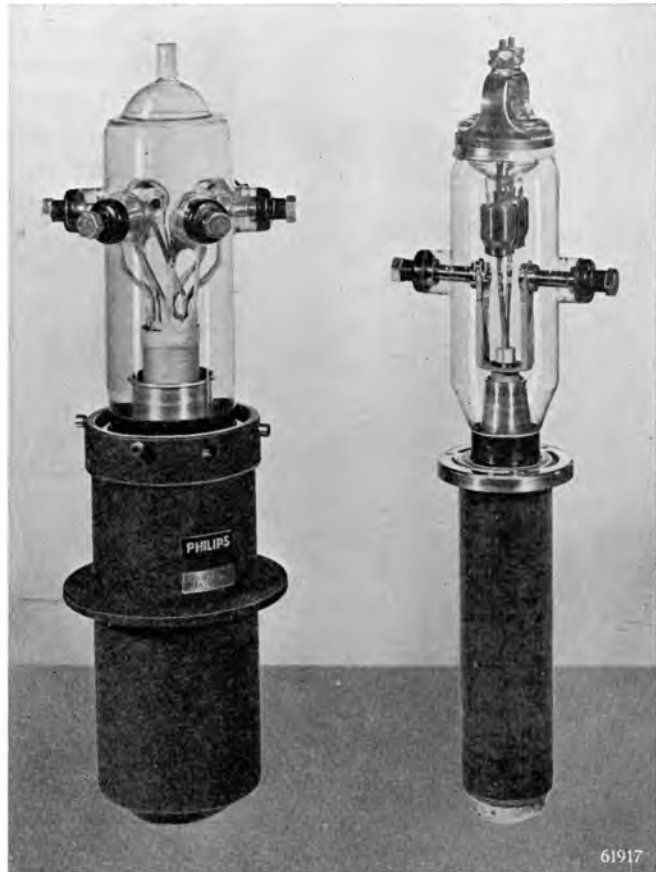
Fig. 2b. Triodes with tungsten heater: TA 12/35 and TAL 12/20. The first has a water-cooled anode, whilst the anode of the TAL 12/20 is air-cooled, the maximum dissipation being 20 kW.
