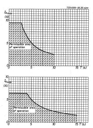
The top curve shows the maximum number of seconds in any 10 second period for which a given average current may be drawn from a sinusoidal supply if the peak voltage applied to the tube is less than 1.25 kV. The bottom curve shows the maximum number of seconds in any 15 second period for which a given average current may be drawn from a sinusoidal supply if the applied peak voltage lies between 1.25 and 1.5 kV.
