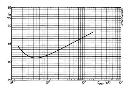
$\begin{array}{l} \mbox{Maintaining voltage under dynamic conditions} \\ \mbox{$C_{par}$ = Capacitance in parallel with tube.} \end{array}$
