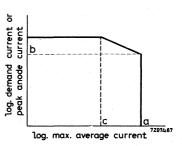
All data assumes full cycle conduction with an equally distributed load on all ignitrons, regardless of whether phase control is used.
