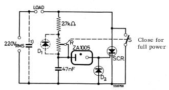
$\mathbf{D_{1}}.$  reduces load of the variable resistor  $\mathbf{R_{S}}$
