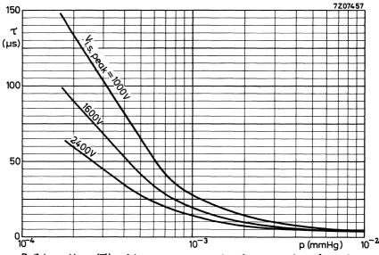
Build-up time ( $\Upsilon$ ) of ion source current pulse as a function of gas pressure(p)
