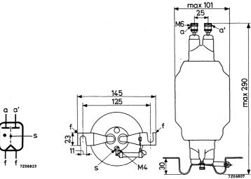
The screen s is connected to the cathode via a resistor.
