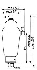
Pins 2 and 3 heater, pin 4 cathode return
