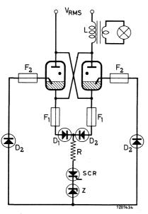
$V_{RMS}$  220 250 380 500 600 V R 2 2 4 5 6  $\Omega$   $F_1$  = 2 A fast response time  $F_2$  = 10 A fast response time
