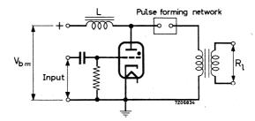
Measured at 5 kV in a typical circuit the time jitter is max. 0.02  $\mu sec.$  Under practical operating conditions the average value of the anode time jitter is about 0.004  $\mu sec.$
