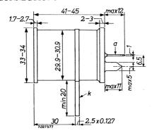
Cathode connector 0.127 mm thick
