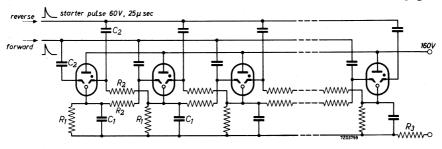
$R_1$  = 10  $k\Omega$  to 33  $k\Omega$  with  $C_1$  = 56 nF to 6.8 nF  $R_2$  = 0.2  $M\Omega$  to 1.2  $M\Omega$  with  $C_2$  = 2 nF to 220 pF  $R_3$  = 6.8  $k\Omega$  to 22  $k\Omega$
