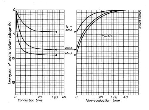
Formation and recovery curves of the starter ignition voltage for a nominal tube
