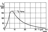
Fig.1c Typical forward peak current through  $10~\Omega$  resistor
