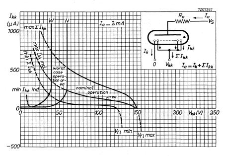
For low cathode selecting voltages the current  $I_{kk}$  to the "off" cathodes will increase and the readability of the "on" cathode will be affected. It is therefore recommended to use a nominal operating point to the right of line N. Under the worst operating conditions the operating point should never reach the area left of line W.
