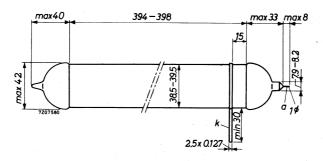
Cathode connector: 0.127 mm thick
