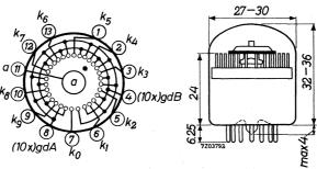
$K_{O}^{\phantom{O}}$  is aligned with pin 7 to within  $\pm\,3^{O}$
