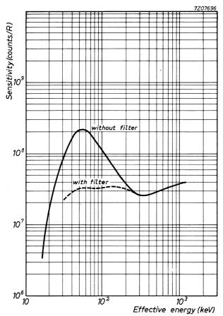
Halogen quenched  $\beta$  (>0.3 MeV) and  $\gamma$  radiation counter tube.
