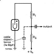
Note: The value of  $R_1$  should not be lower than the value specified by the manufacturer.
