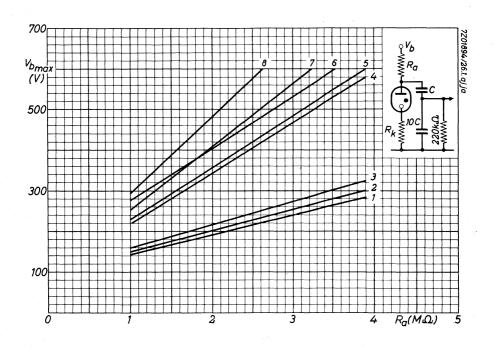
Max. anode supply voltage for self ext. circuits.
