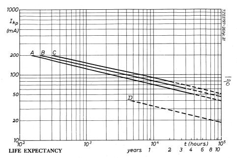
The curves show the life expectancy when the tube is run continuously at room temperature.
