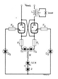
$V_{RMS}$  220 250 380 500 600 V R 2 2 4 5 6  $\Omega$   $F_1$  = 2 A fast response time  $F_2$  = 10 A fast response time Z = zener voltage  $\geq$  18 V
