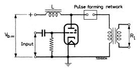
Measured at 3 kV in a typical circuit the time jitter is max. 0.02  $\mu$ sec. Under practical operating conditions the average value of the anodetime jitter is about 0.004  $\mu$ sec.
