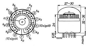
$K_0$  is aligned with pin 7 to within  $\pm 3^{\circ}$
