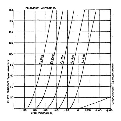
The accompanying curves give the average static characteristics of the No. 242A Vacuum Tube. These curves are taken with the filament operating on alternating current and with the plate and grid returns connected to a center point of the filament transformer.
