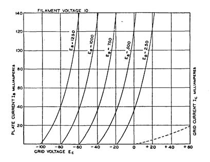
The accompanying curves give the average static characteristics of the No. 276A Vacuum Tube. These curves are taken with the filament operating on alternating current and with the plate and grid returns connected to a center point on the filament transformer.
