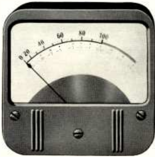
Close up of Volume Indicator Meter, standardized for broadcast use. The upper row of figures shows program level in terms of percentage of optimum transmission requirements. The lower row of figures is calibrated in vu, above and below the 100% reference point.
