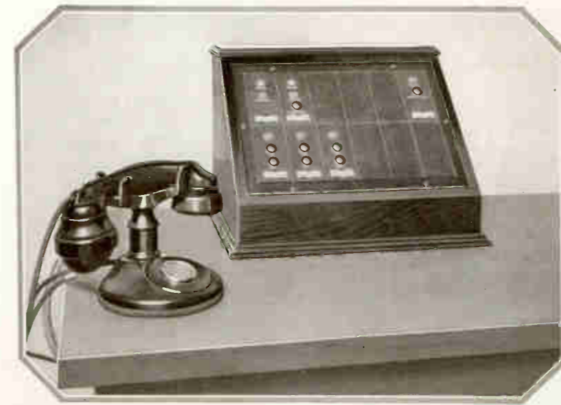
A comprehensive Studio Control System is a part of the No. 8-A and No. 8-B Speech Input Equipments
