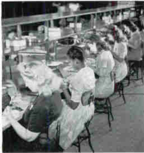
4 Rows of girls assemble the components. Teams of six operators and an inspector carry the assembly through to the finished mount structure.
