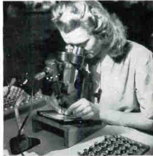
11 Finished mount structures receive a critical inspection under a microscope, then are tested for "shorts" and "opens" before proceeding to next step.
