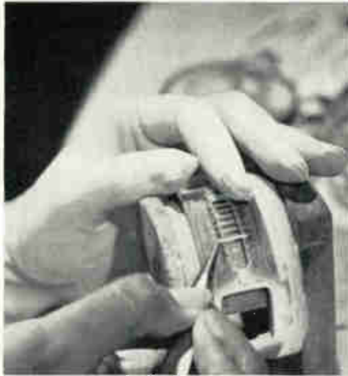
1 Preparation of components is the first step. Here cathode elements, with welding tabs attached, are assembled in a jig prior to spraying.
