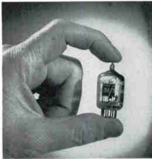
17 A finished miniature tube—manufactured carefully, tested thoroughly and aged properly—ready to go to work in a countless variety of electronic circuits.
