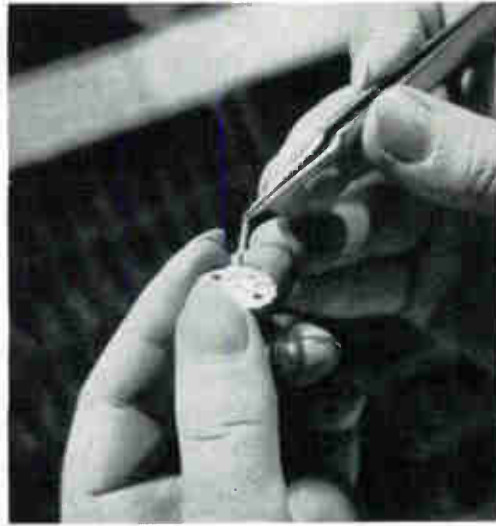
5 Assembling coated cathode on a mica base is the first operation. Deft fingers and a steady hand are required for this and the succeeding operations.
