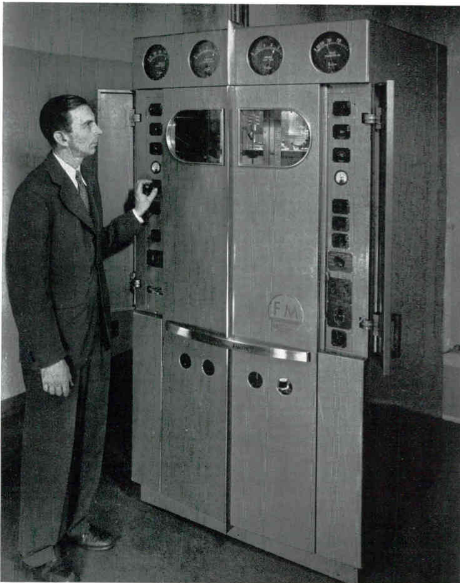
Above: Corson Donaldson, chief engineer, stands beside KUSC's Western Electric FM transmitter, operating on a frequency of 91.7 mc. Transmitter power is 1 kw, licensed effective radiated power is 2.9 kw.
