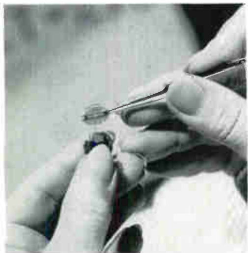
9 Next, the top mica and getter are placed in position. Although the individual parts are fragile, finished structure is extremely rugged.
