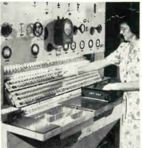
14 Aging miniature tubes on this unique revolving drum insures uniformity and stability in operation. Here, panel is being filled with tubes.
