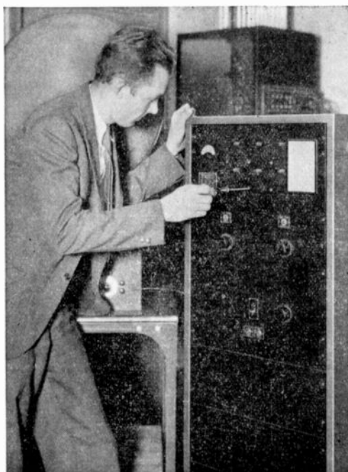
Figure 1, left—The 11B receiver, like the 11A, mounts in the 6A cabinet, which is rugged and self supporting
