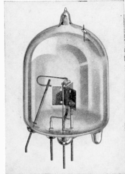
Fig. 10—This tube will oscillate at frequencies up to 740 megacycles. Note the absence of the usual press and the extremely small size of the elements
