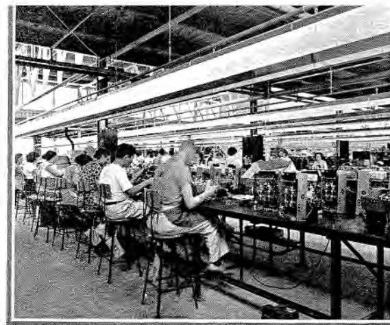
No let-down in intensity occurs along the assembly lines. 150-watt lamps are installed on 30-inch centers.
