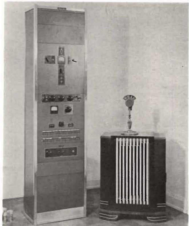
Station speech-input bay, with automatic program amplifier, microphone and monitoring loudspeaker.
