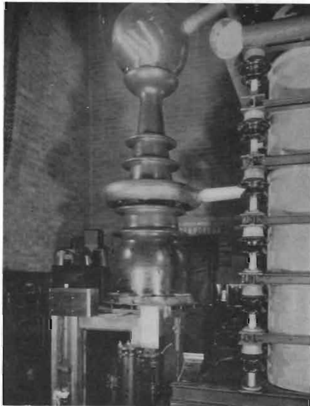
Fig. 1. 600-kv vacuum tube built at Memorial Hospital (New York City) with the cooperation of the W.P.A.
