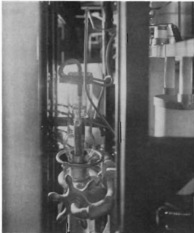
One of the two 100-kilowatt final amplifier power tubes used in the Doherty circuit.
