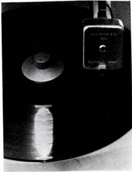
Fig. 2. The frequency characteristic may be measured by means of a light band.
