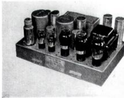
Fig. 4. The 82-A monitoring amplifier (left) as normally furnished, and (right) mounted in a Type 36-A panel shelf.
