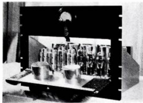
Fig. 3. Several views of the Type 40-D studio amplifier, which includes a built-in floating VI meter. In this type of construction components and tubes are mounted on a hinged subpanel, as may be seen in the bottom view.
