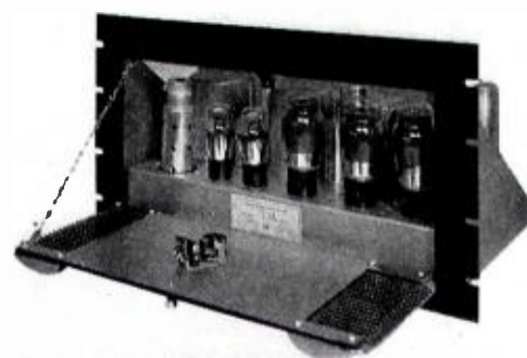
Fig. 4. The 82-A monitoring amplifier (left) as normally furnished, and (right) mounted in a Type 36-A panel shelf.
