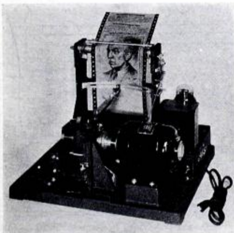
The home facsimile receiver with cover removed.
