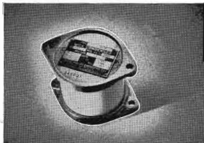
TYPE 59 Mica Transmitting Capacitors. Encased in a ceramic tube with cast aluminum end-terminals. Series, series-parallel or any other combination, can be obtained by bolting terminal ends together. These capacitors are used as neutralizers, padders, in tank circuits and wherever low capacity at high voltages is required.
