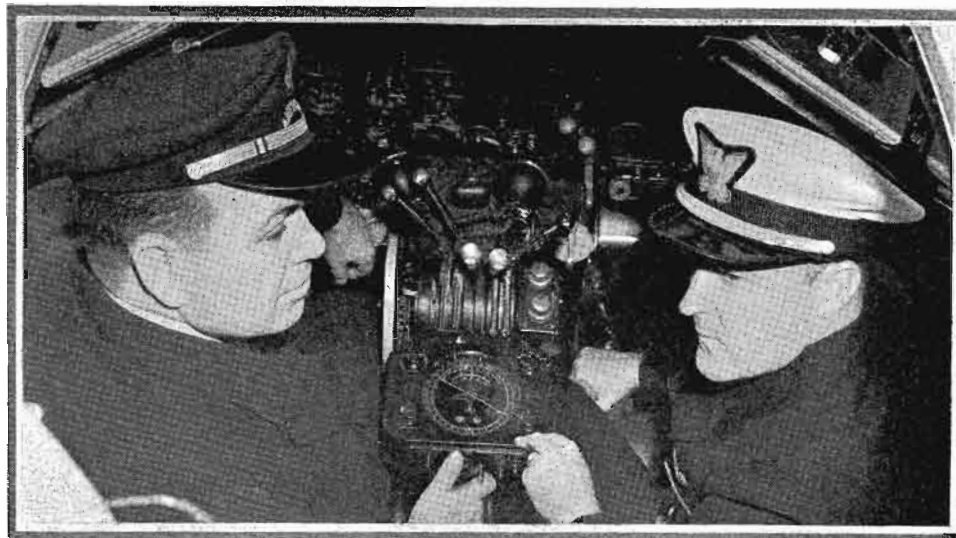
Fig. 1. The automatic direction finder installed in a plane.
