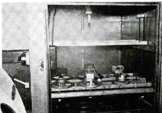
Cinaudagraph Speakers will operate under all climatic conditions. Production line models are spot checked, in a humidity chamber to prove their ability to operate under conditions for which they are designed. Atmosphere in chamber is kept at 98% relative humidity.
