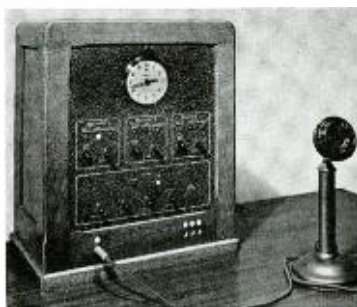
Fig. 8. Closeup of the control turret by which the operator records weather forecasts.
