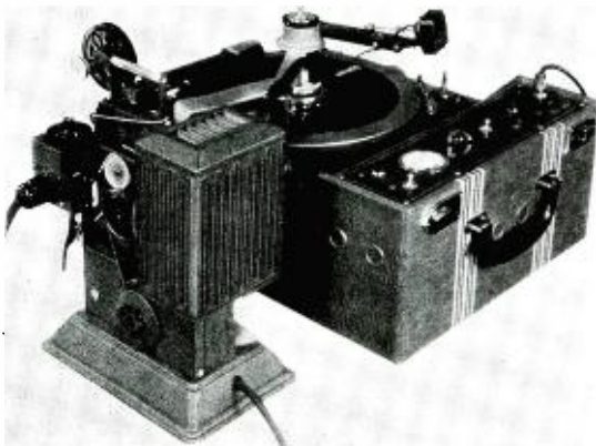
Syncrosound system in use with projector and recorder. The master commutator is mounted on the center shaft of the turntable. The projector commutator is coupled to the shutter shaft.
