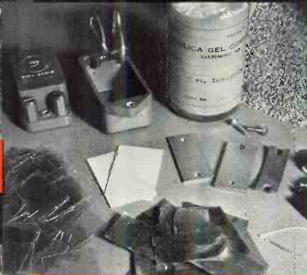
A precision mica condenser in the making: low-loss bakelite case, heavy brass end-plates; heavy spring pressure-plate; selected India mica; tin foil; blotting paper; silica gel; ground cork; Ozite sealing compound; leads; assembly screws
