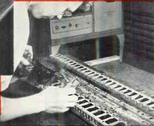
A precision mica condenser in the making: low-loss bakelite case, heavy brass end-plates; heavy spring pressure-plate; selected India mica; tin foil; blotting paper; silica gel; ground cork; Ozite sealing compound; leads; assembly screws
