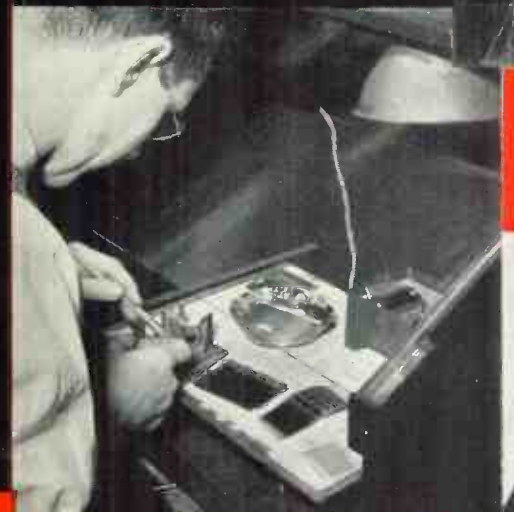
During assembly all parts of the condenser are maintained at 300 degrees F. to drive out all moisture; the workman has a glass shield between his face and the condenser parts both to prevent moisture from his breath reaching the parts and to hold the heat from the electric hot-plate upon which the condensers are assembled
