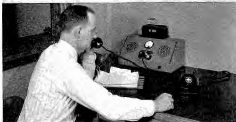
(Top) Desk police officer at headquarters in Maywood, Ill., using two-way f-m units. The transmitter and receiver are located in rear of the desk. (Bottom) Officer at police station in Riverside, Ill., at an f-m remote control unit, for two-way operation.
