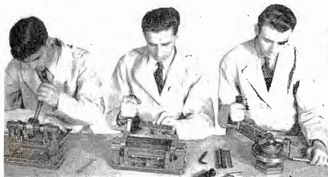
In illustration from left to right: 1st—Di-Acro Shear squares and sizes material, cuts strips, makes slits or notches. 2nd—Di-Acro Brake forms angles, channels or "Vees". 3rd—Di-Acro Bender bends angle, channel, rod, tubing, wire, moulding, strip stock, etc.
