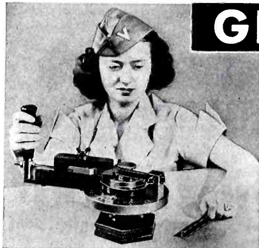
BENDERS — DI-Acro Bender bends angle, channel, rod, tubing, wire, moulding, strip stock, etc., 2 sizes. Capacity up to 1/2" cold rolled steel bar.
