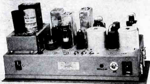
Type PRS-9X, 30-40 MC Mobile Receiver with Dust Cover Removed.
