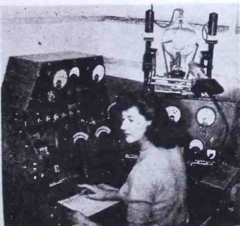
Testing transmitting tubes with the aid of an oscilloscope at the Eimac plant.
