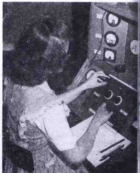
Figures 13 (above) and 14 (below) Figure 13, flashing the getter by high frequency after the tube has been pumped and has had its base attached. Figure 14 checking electrical characteristics and light output on cathode-ray tubes. Preheater at lower right makes preliminary test for short and voltage breakdown.
