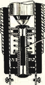
BUILT-IN RESISTOR HOUSED IN SPRING CONTACT EYELET
