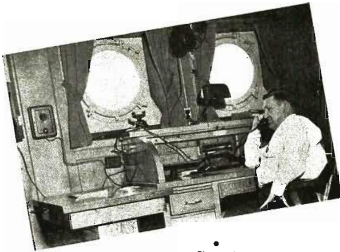
Figure 1 Great Lakes radio communications system in operation. In this installation the cradle-type telephone instrument is linked to the system.
