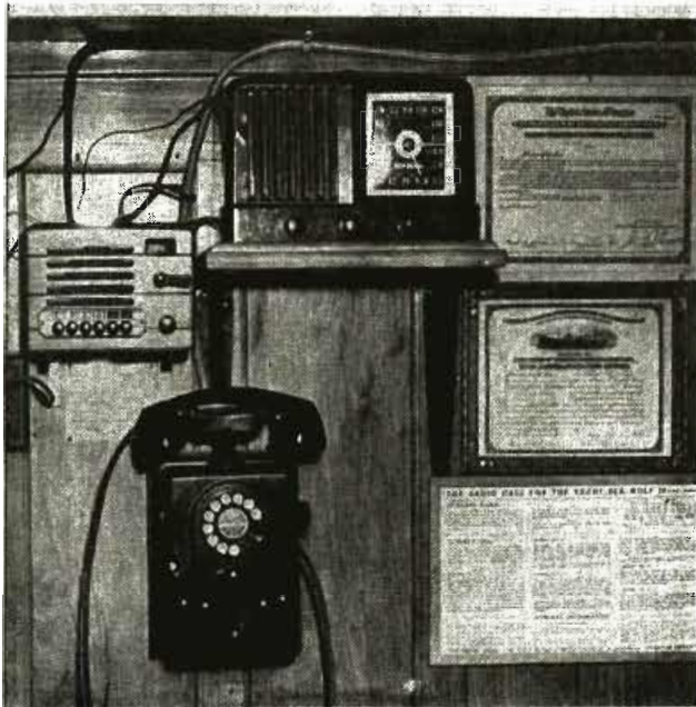
Figure 2 Great Lakes heavy craft radio communications installation, where the telephone instrument and dial system, and miniature speaker are combined in one unit.
