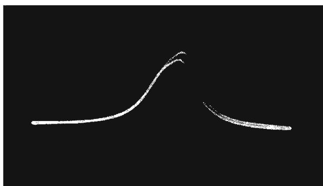
Figures 5 (left) and 6 (above) Figure 5. Trace of the last i-f stage of a television receiver with the sweeper connected to the grid of the last amplifier tube, and an oscilloscope connected to the output of a diode detector. Figure 6. The same trace with the 10-mc mark turned on.
