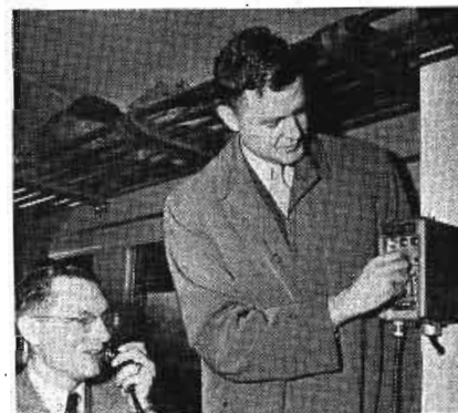
Remote-control unit with loudspeaker and dynamic microphone, inside a Diesel cab.
