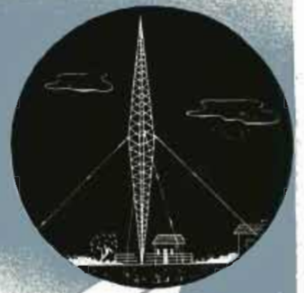
1930 Half-wave vertical radiator, now in general use, was developed into practical form. It greatly improved signal output of broadcast stations.
