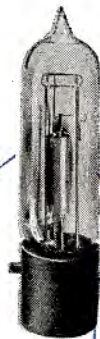
1918. This "peanut" tube, the Western Electric 215A, was developed for service in World War I. It was the first commercial tube whose filament was powered by a single dry cell . . . made possible compact, light weight radio equipment.
