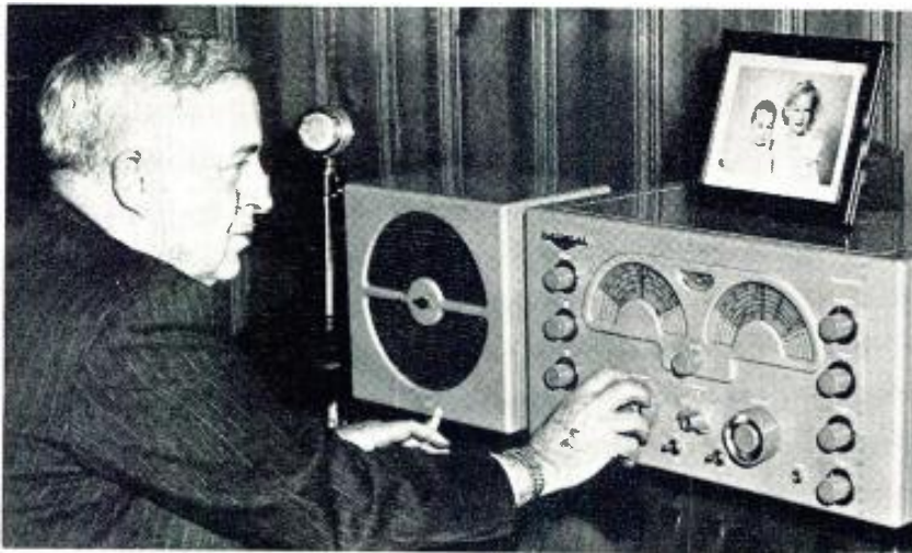
VWOA honorary member William A. Ready, president of the National Company, at the controls of National's communications receiver, NC-173
