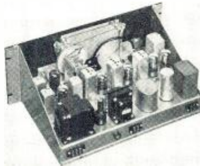
Figures 6 and 7 In Figure 6 (top) appears an interior view of the amplifier and in Figure 6 (below) an underside view. Resistors and mixer crystals are mounted on a terminal strip. The bypass and individual decoupling filters are of the bathtub type and located under the strip, so that the leads from the decoupling resistors pass the terminals of the capacitors and go to the tube sockets without including more than 1" of wire.
