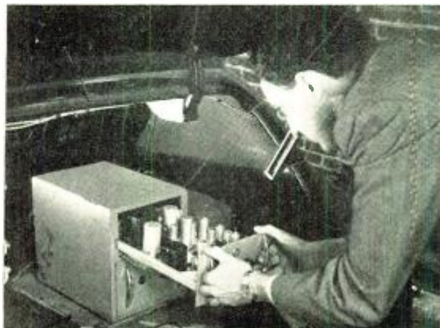
(Right) The 20-watt instantaneous heating Kaar transmitter; FM 175X. FTR taxi receiver, a 14-tube double conversion model.
