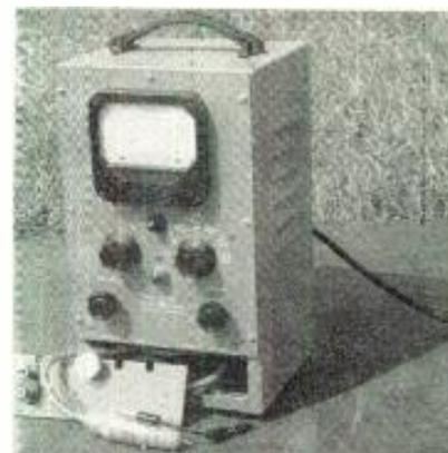
The vtvm used by Eidson (Courtesy Hewlett-Packard).
