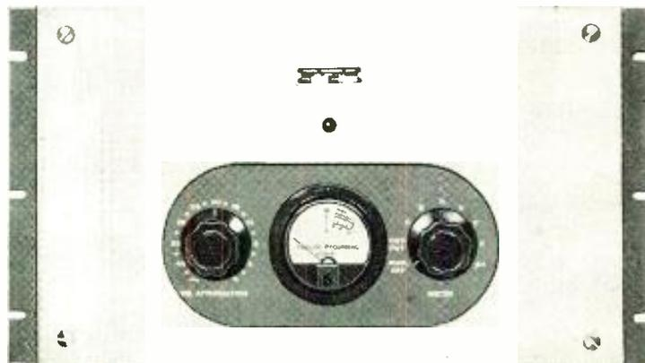
*Type 89A.* Chassis construction is for vertical rack mounting. Removable front panel for easy access to all circuits. Meter and selector switch provide convenient indication of output level at 1000 cps and current readings of all tubes.
