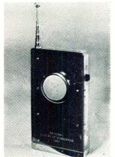
Figure 2 Front view of the 5-tube crystal-control miniature transmitter.
