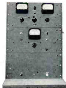
FEDERAL'S TV Monitor meets all FCC requirements. Designed for long service life, it accurately measures video carrier frequency, and monitors sound carrier and modulation.
