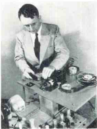
High-speed ( Ultrafax ) transmission via TV was demonstrated recently by RCA in Washington. At left, Donald S. Bond of RCA Labs. placing a strip of film containing outgoing messages in the scanning units of the newly developed system. As the film runs at constant speed through this unit, a pinpoint of light generated in flying spot scanner (lower left) is focused on the film and sweeps across it thousands of times a second. The resulting light impulses are converted into corresponding electrical impulses which are then transmitted.
