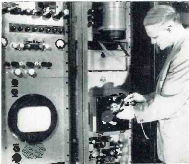
Above: Messages transmitted are reconverted to original form at receiving terminal shown above with C. J. Young of RCA Labs. adjusting the receiving camera. The messages are reproduced as TV images on a kinescope tube in the cylinder at upper right and are copied on film by the camera directly beneath the cylinder. Exposed film is then processed in 45 seconds. Below: Simplified operational schematic of Ultrafax system.
