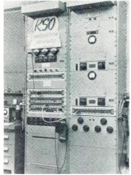
Figure 1 View of the old two-bay speech input equipment with patch panels, auxiliary monitoring amplifiers, two line amplifiers and two microphone preamps plus bridges, pads, four-channel mixer, etc.
